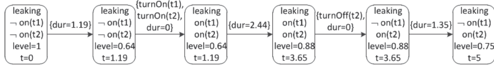
Figure 6.10: A Path in the Transition System of Two Taps Water Tank Example.
